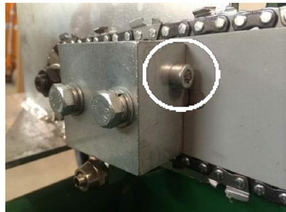
19. Fit the conveyor belt over the bottom roller and assemble the galvanized steel bracket to the bottom of the conveyor using the 8 nuts and bolts provided.
