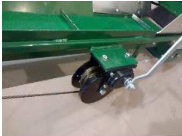
26. Remove the pulley on the operator side of the conveyor, feed the cable through and re-install the pulley.
