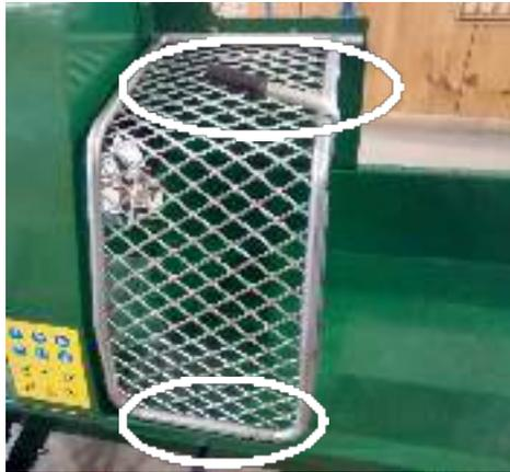
14. Install the larger cage by sliding the pipe into the hole and resting the other side on the bracket. Use the supplied bolt and nut to keep the bar in place so it can freely rotate open and closed.
