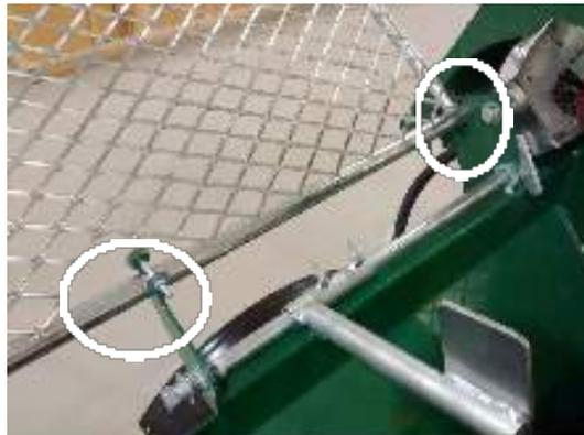
15. Install the notched plate on the processor with the 2 nuts and bolts provided. This plate is used to lock the handle in place which holds the 2/4 way splitter is at the desired height.
