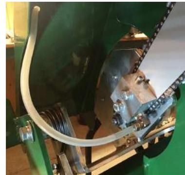
9. Install the back plate, reinforcement bracket, and the top pulley housing to the chainsaw bar guard using the bolts provided. Tighten all bolts including the bolts from step 7.
