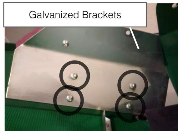
20. With the galvanized bracket now bolted to the conveyor, lift it in place so that it can be attached to the processor. A scissor jack or car jack can be used to aid in lifting the conveyor up into place so the mounting holes align.
