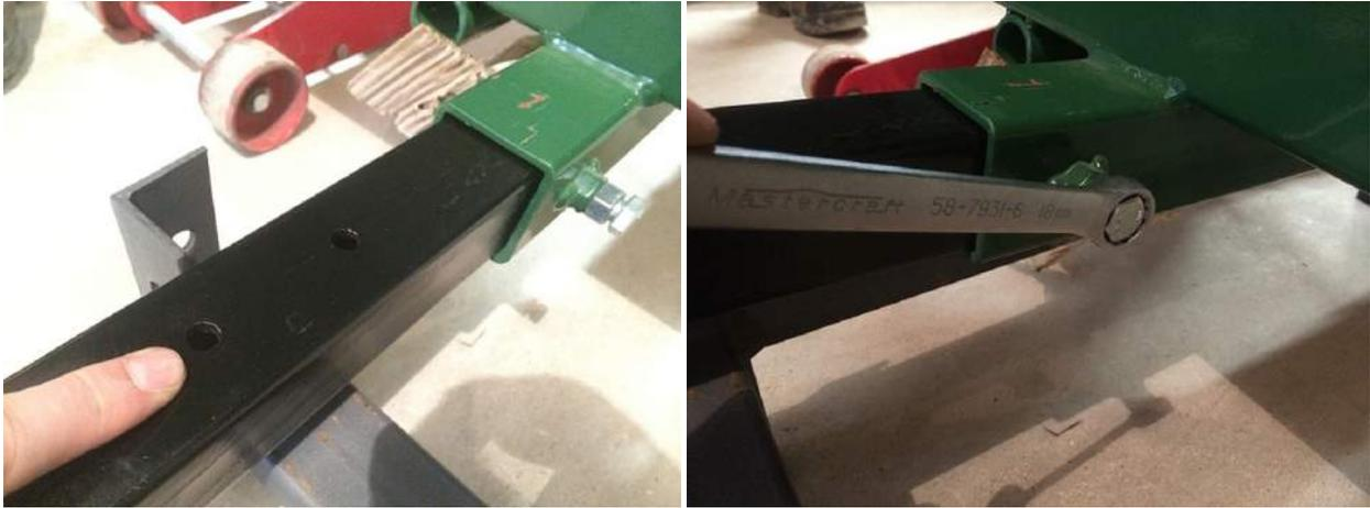
3. Place a liberal amount of grease on the inside of the wheel hubs and in the bearings (or use the grease nipples on the backside of the wheels). Insert greased bearing, washer and nut over axle spindle and tighten the nut. The cotter pin can be inserted into the hole in the end of the axle. Finally, the dust cap can be installed. See below images.
