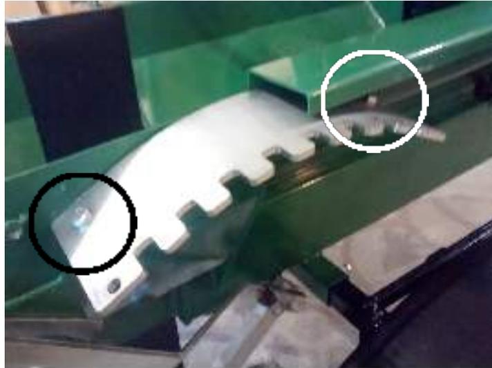
16. Install the 2/4 way splitter bottom support as shown below. The handle can also be installed at this point along with the 2/4 way splitter itself.
