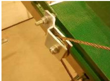
27. Remove the large pulley from the pulley housing on top of the chain guard, feed the cable through and re-install the pulley.
